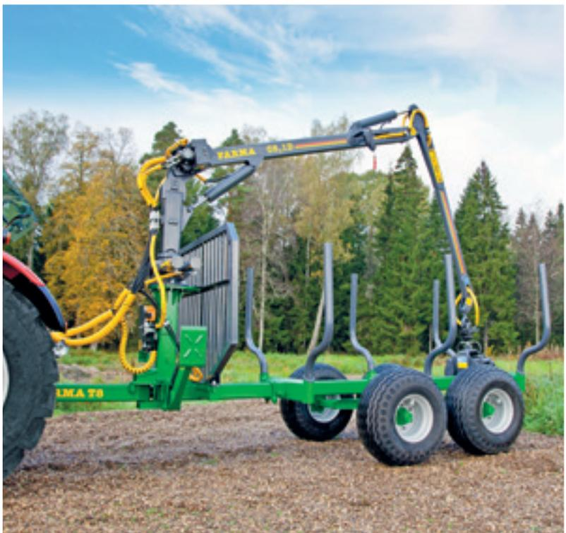
The FARMA CT 5.3-8 lumber trailer is equipped as standard with hydraulic support legs, 3 banks and equipped with 400/60 15.5 wheels. As you can see in the picture, the support legs are well protected in front of the railing while in the up position.
