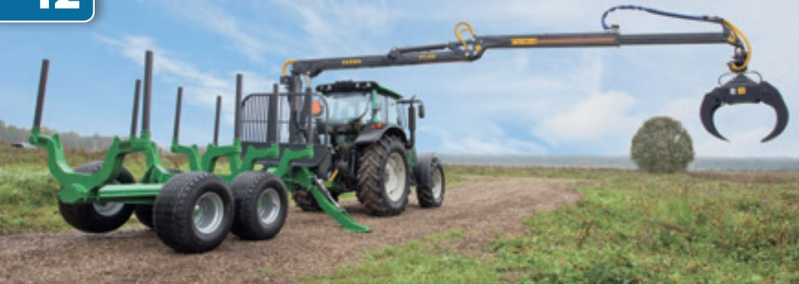
The FARMA C 7.0 is one of the market's most well-thought out and best value-for-money cranes. The crane has a reach of 7.0 m with single extension. The lifting power and movement geometry are exceptional. The attractive design, together with the choice of material, give a low dead weight.
